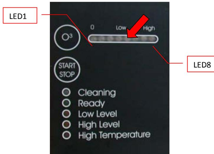
To help check this the blue led bar can be used. To check the level, press-and-release the 'O<sup>3</sup>' button until the blue bar is half full (this way you see when it displays the pressure). Now press-and-hold the 'O<sup>3</sup>' button for 10-15 seconds. The display will start displaying the measured pressure.
