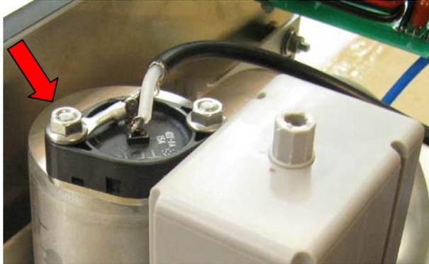
Step 2. Remove nuts from transducer holder and remove holder.
