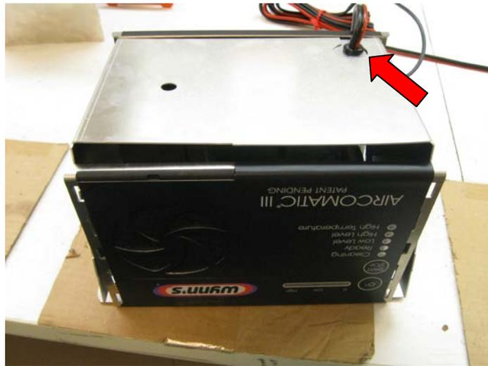
Step 2. Press on the top of the shell to push it into the other shell, please not, make sure that you align the ozonebox with the hole
