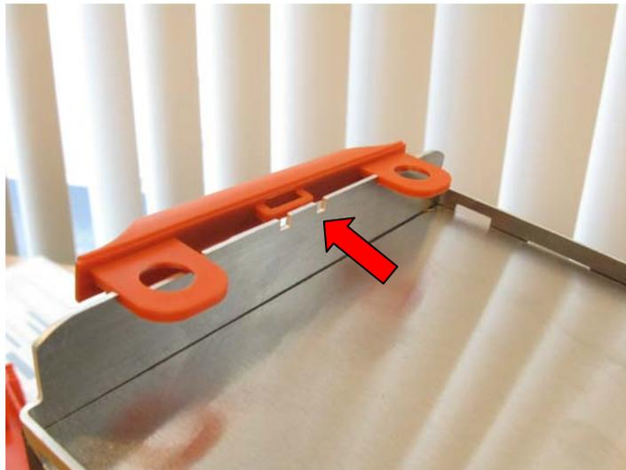
Step 3. Remove the handle, by lifting the it from it lock-position
